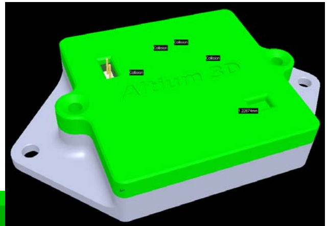
Figure 31. Highlighted 3D body collisions and violations.
